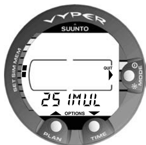
Abb. 4.16 Untermenü Tauchgangs-Simulation. [2 SIMUL].
